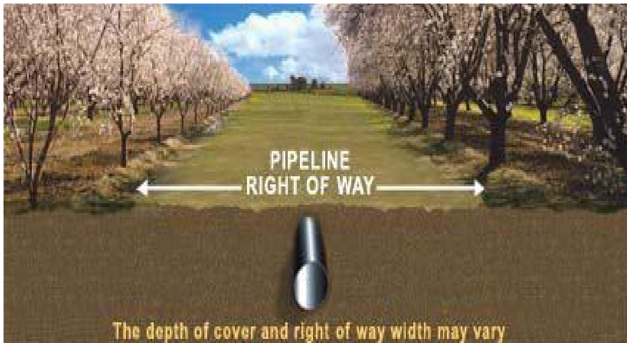
Plate 2: Pipeline Right of Way (PROW)
